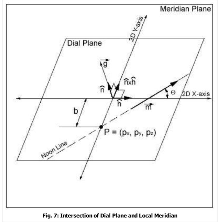
Fig. 7: Intersection of Dial Plane and Local Meridian
