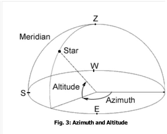
Fig. 3: Azimuth and Altitude
