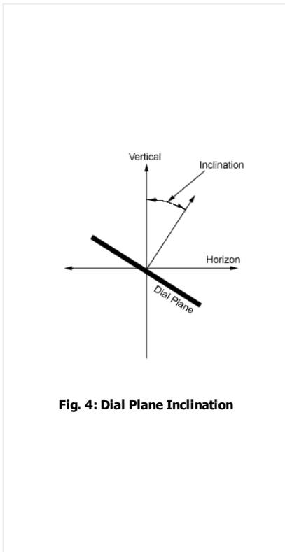
Fig. 4: Dial Plane Inclination
